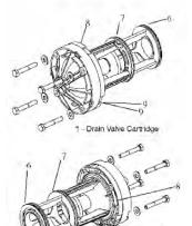
3 - No Hard Water Bypass Valve Cartridge
